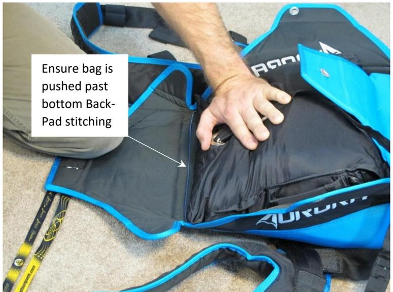
**Step 11.** Close bottom and top flap as usual. Note position of Velcro on bridle. Bridle **must** come out from the bottom!
