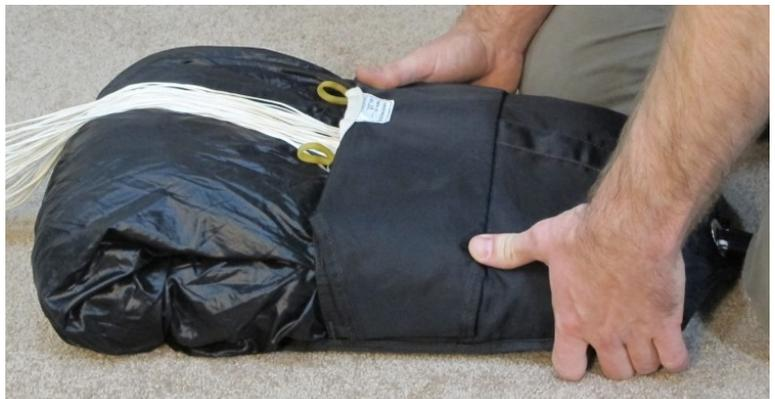
**Step 6.** Stand D-bag up, fold/roll remaining canopy fabric into bag as shown. ↓→
