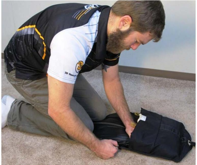
**Step 4.** Make first stacking S-fold no greater than half the length of the bag.
