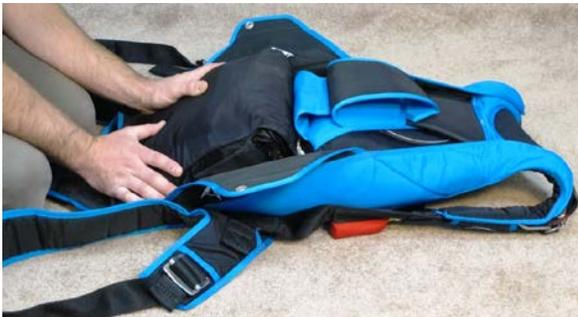
**Note:** Main closing loop should be no longer than 1 1/2" (30mm). **38 mm**
