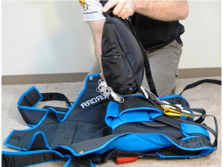
**Step 10.** Attach pull-up-cord to closing loop. Center the bag in the main pack tray and press it deeply into container.
