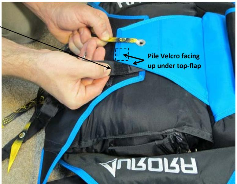
**Step 12.** Before pulling side-flap closed, thread pull-up cord, then **firmly** push the bottom corner tab under the bag.
